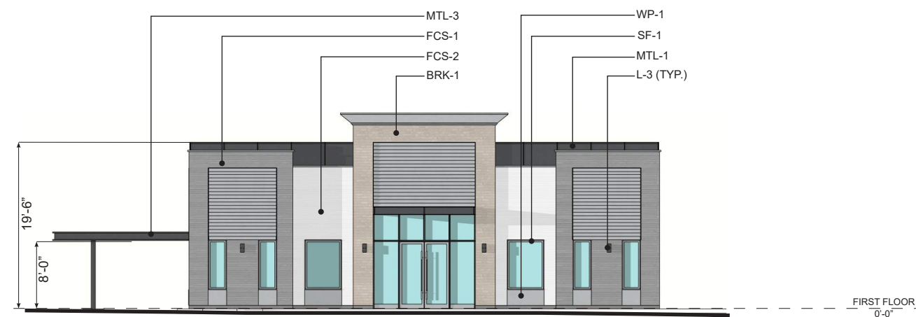
2 NORTH EXTERIOR ELEVATION SCALE: 1/8" = 1'-0"
